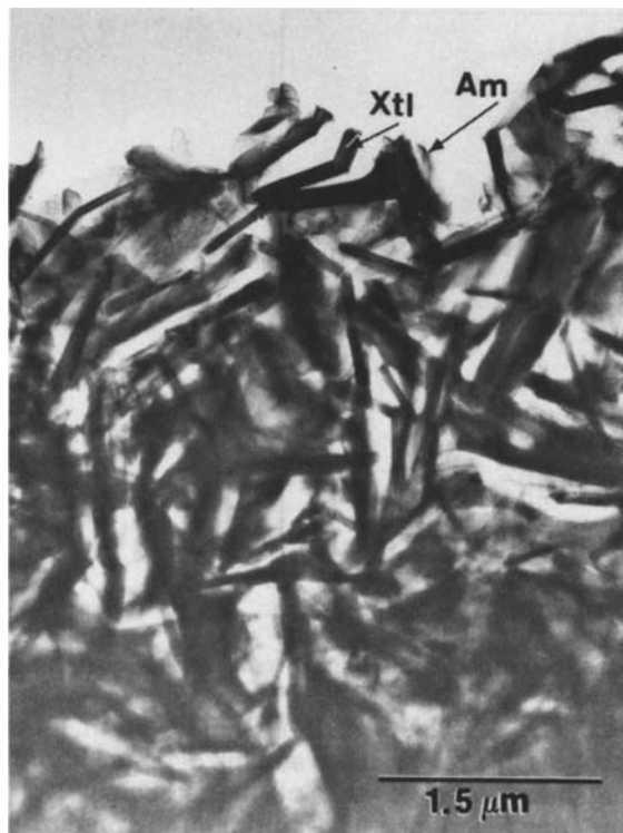
Figure 3 TEM micrograph of an area of hot-pressed BN-binder showing acicular crystals.
