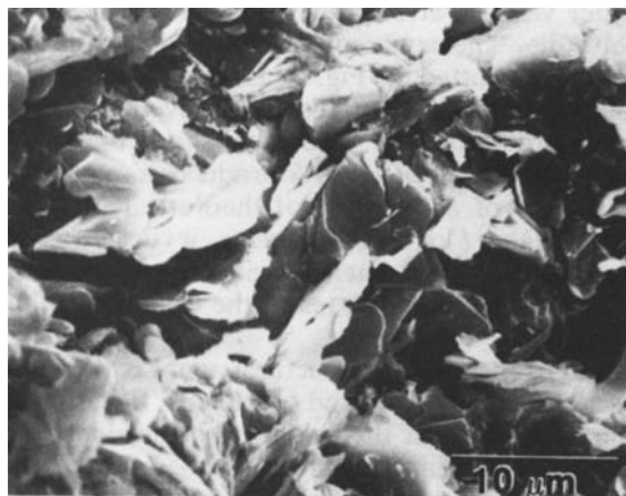
Figure 4 Micrograph of fracture surface of a hot-pressed BN-binder composite showing intergranular fracture and platelike grains.
